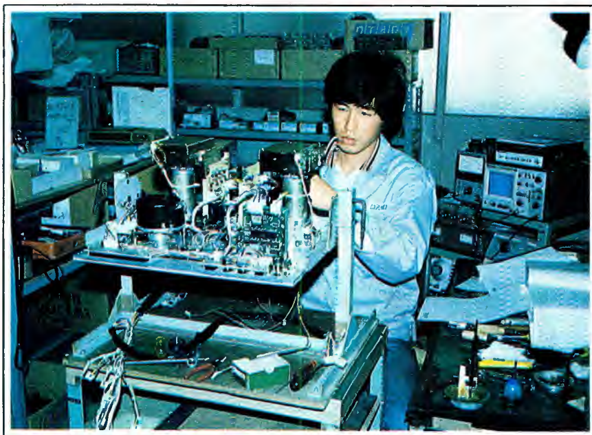
Adjustments are made to the MTR-10 mainframe.
