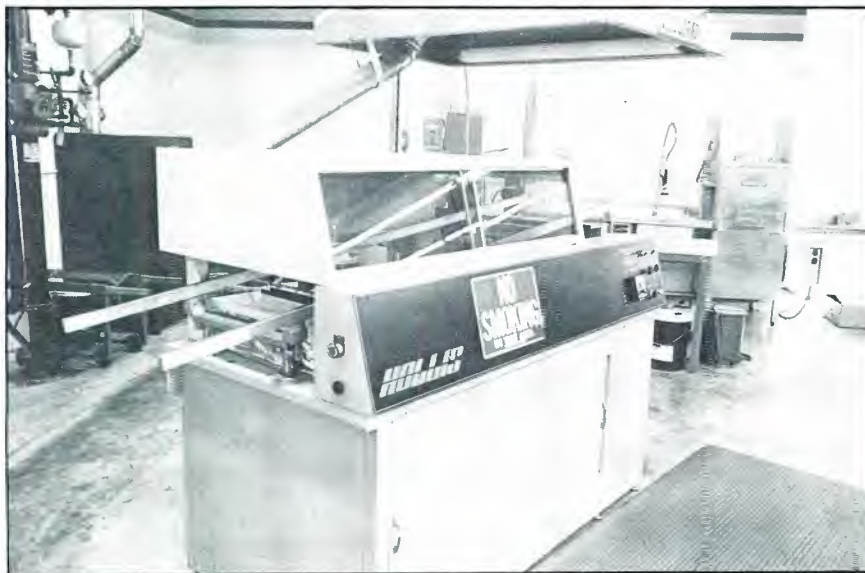
Shown below is an automatic solder wave machine with a washing machine in the background.
