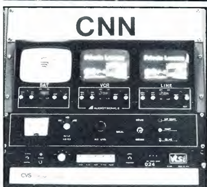
(C) Equipment (at left) for one channel includes video monitors for satellite, VCR and line; the status panel, with audio metering and selection switch; the automatic commercial insertion unit; and the time base correction unit.
