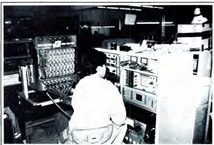
An MX-5050B Mark III-8 set up for final amplifier performance checks.
